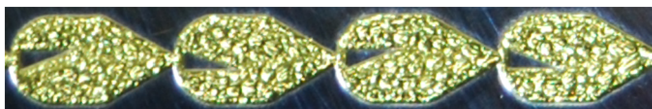
Figure 1. FlowPlate® LL-Triangle-Structure that shows a desirable drop-flow regime.
