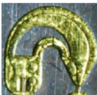
Figure 2. A typical unwanted Parallel-Flow pattern where the denser phase remains close to the wall due to centrifugal forces.
